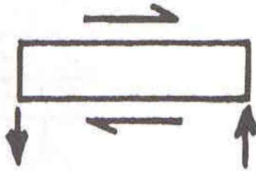
Fig. 8b Restraining couple from columns
